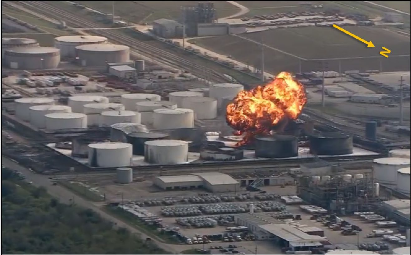
Figure 15. Tank 80-5 flare-up that occurred on March 20, 2019. (Credit: “Raw video ITC fire reignites in Deer Park”, annotations by CSB)
